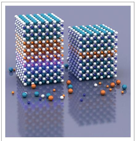
**Figure 1.** Models of heterostructures of lanthanum aluminate between strontium titanate layers. The atoms are represented by colored spheres (oxygen, white; lanthanum, orange; aluminum, yellow; strontium, large blue; and titanium, small dark blue). Image courtesy of J. Huijben, Nymus 3D.
