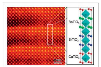
Figure 3. Cross-sectional high resolution transmission electron microscope image of an asymmetric three-component (or "tricolor") superlattice containing (Ca, Sr, Ba) TiO<sub>3</sub>.48
