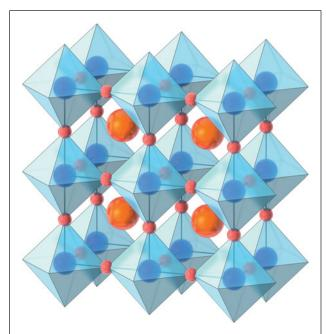
Figure 2. Schematic of the perovskite structure: orange spheres indicate the so-called A-site where A = La, Sr, Ba, and Ca, the blue spheres indicate the B-site, where B = Ti, V, Ni, and Al, and the red spheres indicate the oxygen anion forming octahedra (transparent blue) surrounding the B atom.
