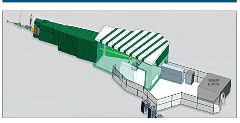
Schematic representation of the VENUS instrument, providing time-of-flight neutron imaging capabilities, at the US Department of Energy's Oak Ridge National Laboratory (ORNL) in Tennessee. Credit: Jill Hemman, ORNL.
