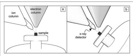
**Figure 1.** Typical dual platform geometry of a focused ion beam scanning electron microscope (FIB-SEM) instrument. (a) SEM imaging configuration and (b) FIB milling configuration with sample surface normal to the ion beam. FIB-SEM instruments are often equipped with additional analytical detectors such as an x-ray detector, as shown here. Adapted with permission from Reference 4.
