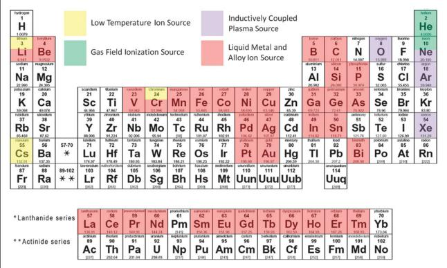
Figure 2. Current and development-phase ion sources by various source technologies encompass a substantial part of the periodic table.
