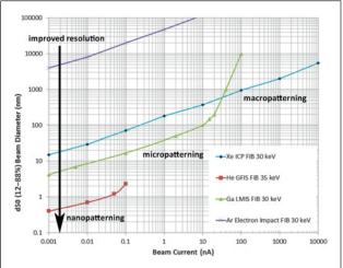
**Figure 3.** Beam size versus beam current graph of ions from different ion sources. Adapted from data courtesy of Noel Smith, personal communication.
