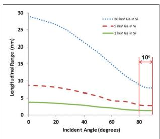
**Figure 6.** A graph of longitudinal ion range of Ga<sup>+</sup> into Si versus incident angle for 30 keV, 5 keV, and 1 keV ions from data using the SRIM (stopping and range of ions in matter) simulation software.<sup>55</sup>
