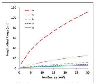
**Figure 5.** A graph of longitudinal ion range into Si at 85° incident angle versus ion energy for common commercial FIB ions obtained using stopping and range of ions in matter.<sup>55</sup>
