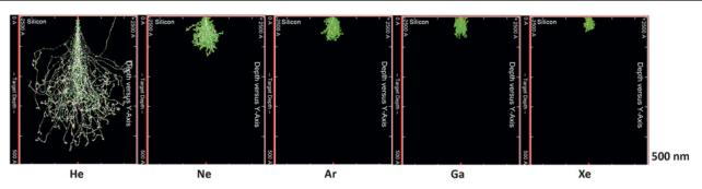
Figure 4. Stopping and range of ions in matter ion trajectories and recoil motion for 30 keV ions in Si.55 The vertical full scale = 500 nm.
