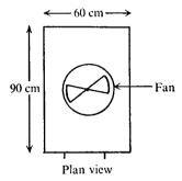
Fig. 1. Diagram of the chamber used to measure the attraction of skin scales onto administration set connector needles and other materials.
