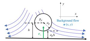
Figure 1. Schematic of a particle at  $(x_p, y_p)$  near a flat wall submerged in an arbitrary background flow **u**.
