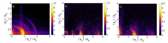
Figure 5. (a) Fourier spectra of electromagnetic waves, (b) electron plasma waves – charge density, and (c) ion acoustic waves in the quarter critical density region for the laser pulse time  $t_p = 0$  and the simulation time t = 5 ps. Color bars are in logarithmic units.
