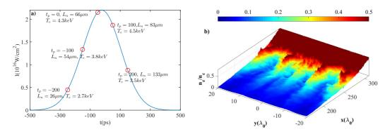
Figure 1. (a) The pulse shape and the selected representative points for the kinetic simulations. (b) Typical filamentation structure observed in our simulations and represented by the electron density distribution at the time corresponding to the laser pulse maximum in panel (a).
