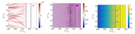
Figure 7. (a) Spatial distribution of the Poynting vector (x-component in W/cm<sup>2</sup>) in real space around the critical density, (b) the charge density  $(Zn_i - n_e)/n_c$  and (c) the ion density normalized to the critical density  $Zn_i/n_c$  for the laser pulse time  $t_p = 0$  and the simulation time t = 5 ps. The solid black lines represent the region  $(0.9 - 1)n_c$  near the critical density.
