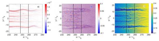
Figure 6. (a) Distribution of the Poynting vector (x-component in W/cm<sup>2</sup>) in real space around quarter critical density, (b) the charge density  $(Zn_i - n_e)/n_c$  and (c) the ion density normalized to the critical density  $Zn_i/n_c$  for the laser pulse time  $t_p = 0$  and the simulation time t = 5 ps. The solid black lines represent the density range between  $0.22n_c$  and  $0.28n_c$  on the initial density profile.
