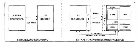
Figure 1. S2 Baseband Processing System Overview. Baseband digitized data are recorded on the S2 recorder at up to 128 Mb/s. S2 tapes are shipped to the processing center, where data are transferred to computer via the S2 Tape-to-Computer Interface (TCI) at up to 16 MB/s, with subsequent processing in software. Note: CIC ('Computer Interface Card') and DMAC ('DMA Card') are additional items to standard S2 and computer systems, respectively.
