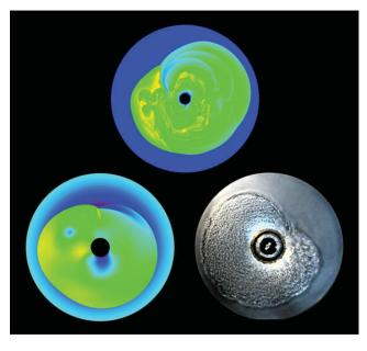
**Figure 3.** The shape of the rotating hydraulic jump observed in the nonlinear regime in the SWASI experiment (right) is similar to the shape observed in the shallow water approximation (left) and the shape of the SASI in the numerical simulations of cylindrical gas accretion with local neutrino cooling (top).
