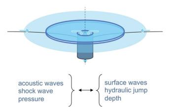
**Figure 4.** Water is injected inward from a circular slit, in a uniform and stationary manner. A circular hydraulic jump is produced by the vertical surface of the cylinder at the centre. Water is evacuated by spilling over the upper edge of this cylinder.
