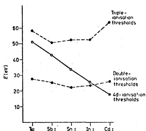
**Fig.4** - Plot of the double- and triple-ionization thresholds and of the 4d-ionization threshold against Z from Z = 48 to Z = 52. Note the crossing at In I. Experimental  $\bullet$   $\circ$  adjusted Hartree-Fock.
