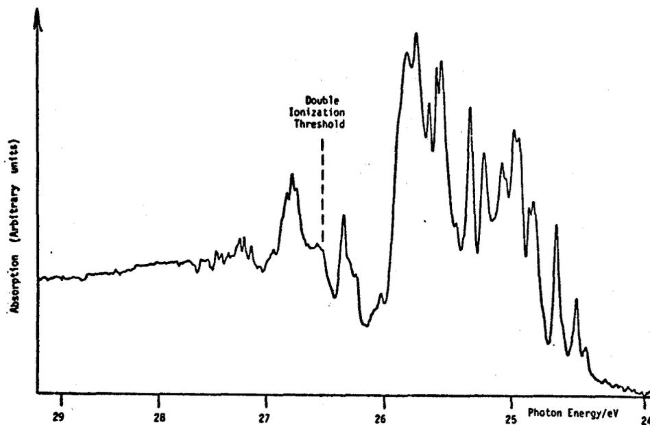
FIG.1. Showing the 'quenching' of 3d — np transitions as the double ionization threshold is passed towards higher energies in Ga I.
