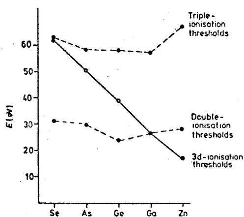
**Fig.3** - Plot of the double- and triple-ionization thresholds and of the 3d-ionization threshold against Z from Z = 34 to Z = 30. Note the crossing at Ga. Experimental  $\bullet$   $\circ$  adjusted Hartree-Fock (see text).
