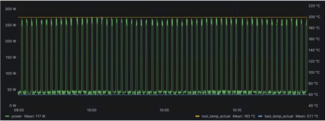
Figure 5. Excerpt of the live dashboards, displaying the temperatures (yellow, blue) and power consumption (green)
