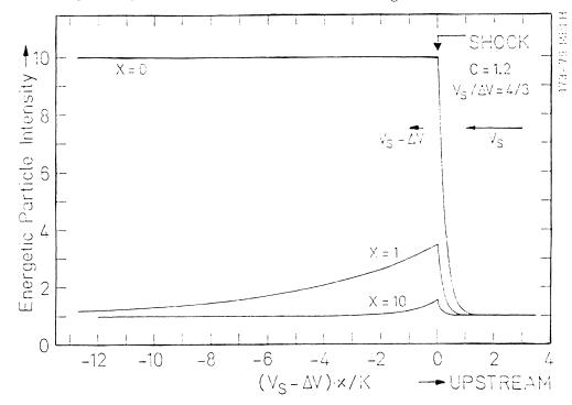
Figure: Relative intensity vs distance in units of  $\kappa/V_s - \Delta V$ ) near a strong shock. A power law source  $\sim p^{-3C}$  is assumed. X =  $4\kappa/V_s^2 \tau$ , for various uniform loss rates  $1/\tau$ .
