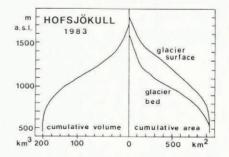
Fig.12. Area and volume distribution with elevation, for Hofsjökull.
