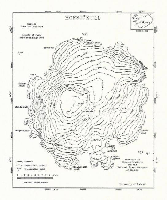
Fig.9. A map of ice-surface contours of Hofsjökull.
