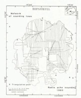
Fig.8. Radio echo-sounding lines on Hofsjökull.
