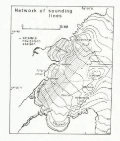
Fig.5. Radio echo-sounding lines on western Vatnajökull, plotted on the map surveyed by the Danish Geodetic Institute in 1937-38.
