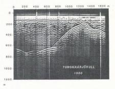
Fig.2. A typical radio echo-sounding profile from Vatnajökull.
