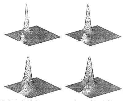
Fig. 9. Probability densities for nonresonant two-mode case; origin at the leftmost corner;  $A_1$  and  $A_2$  axes upward and downward, resp.; increasing noise level from left to right and top to bottom.
