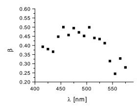
**Figure 2.** Analysis of the time-resolved PL from super bright LED. The stretching parameter  $\beta$  is clearly wavelength dependent. The stretching parameter is largest at the PL maximum of 480 nm and decreases on both the high and low energy sides of the spectra.
