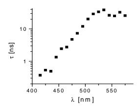
**Figure 3.** Analysis of the time-resolved PL from super bright LED. The stretched exponential lifetime is observed to dramatically increase as the emission wavelength is varied from 420 to 500 nm. The PL maximum is at 480 nm.
