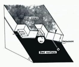
Fig. 2. Cross-slope and down-slope orientation of shear frame at crown of snow slab.
