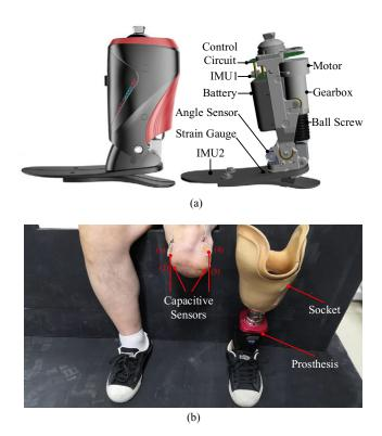
*Figure 1.* The designed robotic transibil prosthesis and wearing diagram. (a) The designed robotic transtibil prosthesis includes the mechanical, sensing, and actuation components. (b) The wearing diagram. Four capacitive sensors (labeled by 1, 2, 3, and 4) are placed on the residual limb.
