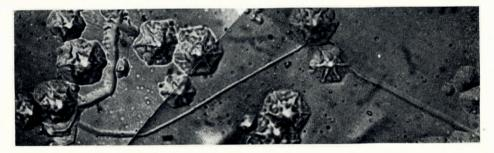
Fig. 7. Channels deflected in the vicinity of etch pits  $(\times 1,000)$
