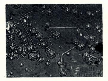
Fig. 6. Channels deflected in the vicinity of etch pits  $(\times 500)$
