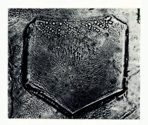
Fig. 2. Inclined section of rows of etch pits in a stressed crystal  $(\times 150)$
