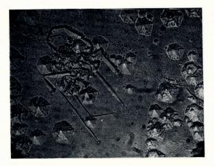
Fig. 8. Channels radiating from a centre of deformation  $(\times 500)$
