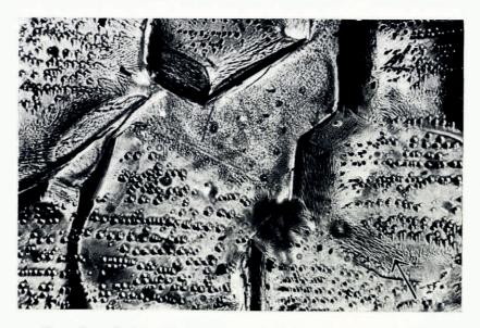
Fig. 1. Rows of etch pits in a stressed crystal. Stress axis in direction of arrow (×200)
