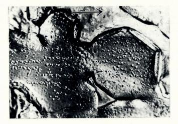
Fig. 3. Rows of etch pits formed without external stressing. Growth direction shown by arrow  $(\times 120)$
