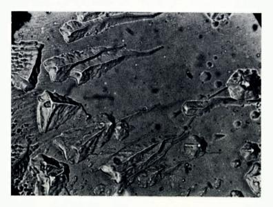
Fig. 4. Tapering etch channels in  $\langle 11\overline{2}0 \rangle$  and  $\langle 10\overline{1}0 \rangle$  directions (×1,000)
