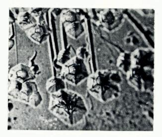
Fig. 5. Non-tapering channels in  $\langle 11\overline{2}0 \rangle$  direction (×1,000)
