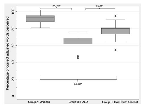
**Fig. 3.** Comparison of percentage of adjusted correct words perceived in the modified rhyme test among the 3 groups where the speakers were (A) unmasked, (B) wearing the HALO device, or (C) wearing the HALO device with a wireless communication headset.
