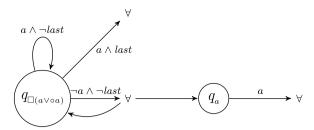
Fig. 2. AFW accepting the LTL<sub>f</sub>-models of  $\Box(a \vee \bigcirc a)$ .
