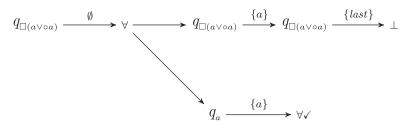
Fig. 4. A run of the AFW of Figure 2 rejecting the input  $\emptyset \cdot \{a\} \cdot \{last\}$ .
