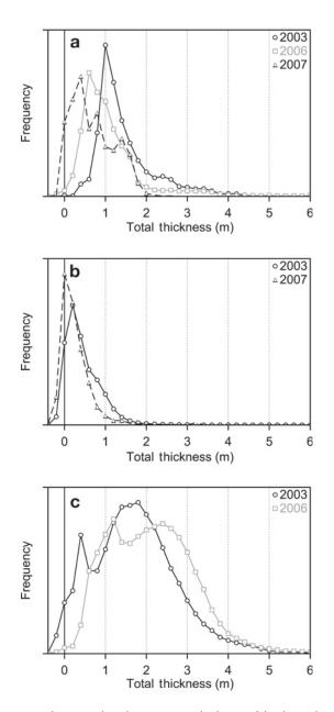
**Fig. 5.** Distributions of total (ice + snow) thickness of the three classes in Storfjorden: (a) fast ice, (b) locally formed ice and (c) advected external sea ice. The histogram bin size is 20 cm. Negative thicknesses arise due to noise and instrument calibration errors.
