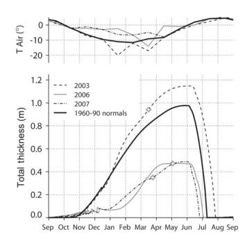
**Fig. 6.** Total ice thickness (bottom) from a thermodynamic sea-ice model (1DICE) representative for the western Barents Sea. Markers indicate the model thickness results at the dates of the surveys. The model was forced with monthly averaged precipitation and airtemperature data (top) from the weather station on Hopen.
