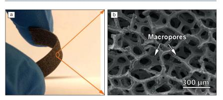
(a) Optical and (b) scanning electron microscope image of the 2D nickel/iron metal-organic framework. Courtesy of Nature Publishing Group.
