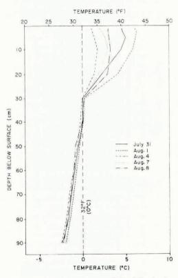
Fig. 2. Sub-surface temperatures, Radstock Bay beach.
