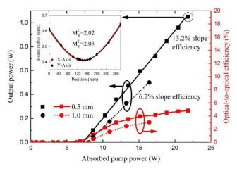
**Figure 6.** Output power of a Tm:YAG disk laser versus absorbed pump power for 0.5 and 1 mm thickness of gain medium. The inset shows the measured beam caustic and calculated beam quality at the output power of 1.05 W.
