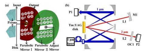
Figure 3. Layout of the (a) 20-pass pumping head and (b) 2 µm Tm:YAG disk laser multi-pass pumped by a 1 µm laser.
