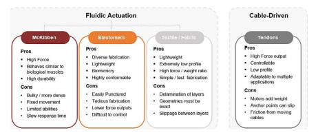
Figure 3. Brief overview of different actuation methods used in soft exosuits and the benefits/disadvantages of the listed types.
