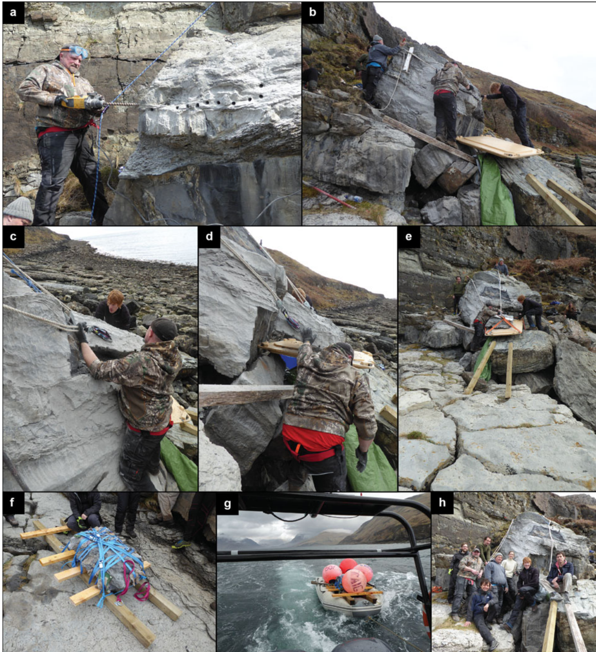
Figure 3 The process of extracting the dinosaur-bearing block: (a) the area of interest was supported by expanding eye bolts attached to a static anchor by slings, and a series of 25 mm diameter holes were drilled around this area; (b), plug-and-feather steel expanding wedges were inserted into the drill holes and struck with hammers in order to propagate cracks that separated the block from the rest of the pinnacle; (c–e) the detached block was lowered to the next level using a ratchet winch, and guided onto a board on a ramp constructed from 100 mm fencing posts onto the limestone pavement beneath; (f) the block was then secured to a wooden cradle by ratchet straps and carried over the beach to be loaded onto a rigid inflatable dinghy, which was towed (g) through Loch Scavaig to the landing jetty at Elgol; (h) the excavation team, from left to right: Roger Close, Brett Crawford, Stig Walsh (top), Andrzej Wolniewicz (bottom), Matt Fair, Elsa Panciroli, Richard Butler and Roger Benson. Photographs a–g by Elsa Panciroli.
