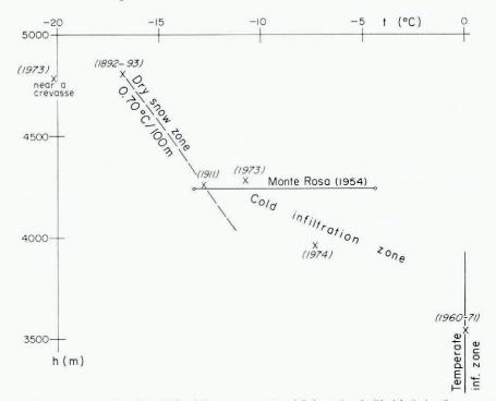
Fig. 3. 15 m deep temperatures found by Vallot (1892–93, 1911) and Laboratoire de Glaciologie (1960–71, 1973, 1974) versus altitude. The horizontal line corresponds to the various temperatures measured by Fisher (1955) on Monte Rosa at larger depths.
