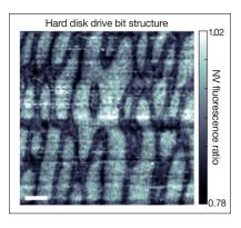
Nitrogen-vacancy (NV) magnetometry image of the bits of a hard disk at T = 6 K. Dark features correspond to the 5.3 G magnetic field contours (2892 MHz RF field). Scale bar, 100 nm. Credit: *Nature Nanotechnology.*
