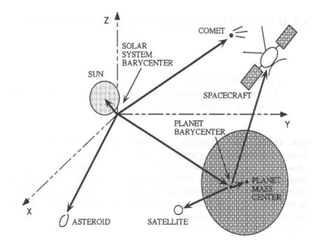
Figure 1. Examples of cartesian state vectors available from SPICE SPK files.
