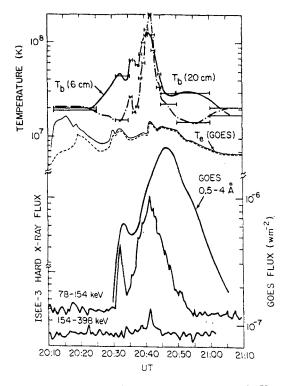
Fig. 5. The time profiles of the 2 and 6 cm peak brightness temperatures, the X-ray electron temperature deduced from the fluxes in two GOES soft-X-ray bands, the flux in one of the GOES bands, and the hard X-ray fluxes in two of the channels of the ISEE-3 spectrometer.
