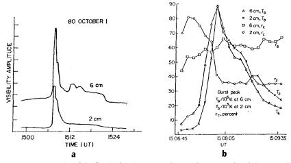
Fig. 1. (a) The time profile of the flux in the shortest spacings at the VLA at 2 and 6 cm wavelengths.(b) The time profiles of the maximum brightness temperatures in the 2 and 6 cm maps during the peak of the burst in (a), together with the variation of the degree of circular polarization at both wavelengths.
