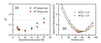
**Figure 5.** (a) The measured  $M^2$ -factor of the Ho:YAG SCF laser ( $T_{oc} = 92\%$ ) at different absorbed pump powers and (b) a typical  $M^2$  measurement at 7 W output laser power.
