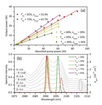
**Figure 2.** (a) Laser performance of the Ho:YAG SCF laser with different OCs and (b) the corresponding optical spectra. The gray curves are the calculated gain spectra of Ho:YAG<sup>[17]</sup> with different population inversion parameters  $\beta$ .
