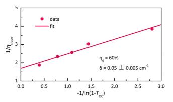
**Figure 3.** Caird plot for the high-power Ho:YAG SCF laser: inverse slope efficiency with respect to the inverse output-coupling loss, i.e.,  $-\ln(1-T_{\rm oc})$ .
