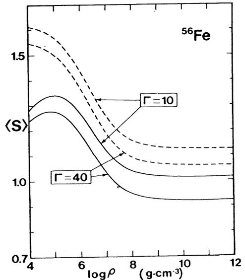
FIG.3. Comparison of Yakovlev and Urpin's resistivity(dashed curves) with present results(solid curves) for the <sup>56</sup>Fe matter.
