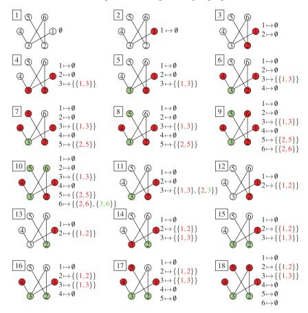
Fig. 1. Graph coloring with backjumping.
