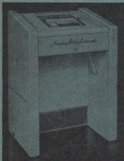
The E.M.40 Clinical Model has facilities for Air and Bone Conduction Tests with pure tones . . . Speech Tests both live and recorded . . . Loudness Balance (Fowler-recruitment) Tests . . . and Masking Tests. Masking is effected with a "white" noise, which can also be used for the new tests devised by Prof. Langenbeck. Click-less tone interruption is provided. Discrete frequencies—from 64 to 1024 c/s at octave intervals, and from 1024 to 11584 c/s at half-octave intervals—may be selected.
