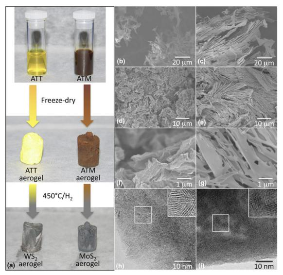
FIG. 9. (a) Synthesis scheme for  $MoS_2$  and  $WS_2$  aerogels. SEM images of (b) ATM, (c) ATT, (d and f)  $MoS_2$ , and (e and g)  $WS_2$  aerogels. TEM images of (h)  $MoS_2$  and (i)  $WS_2$  aerogels. The inset in images (h) and (i) is the magnification of the white box and is 10 nm in width. Reproduced by permission from Ref. 18 (American Chemical Society).
