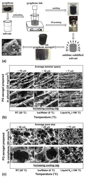
FIG. 11. (a) Schematic of the RTFG process. (b, c) SEM images of (b) phenol-based and (c) camphene-based aerogel structures cooled using liquid  $N_2$ , an ice/water mixture, and at room temperature. Reproduced by permission from Ref. 144 (Wiley and Sons).
