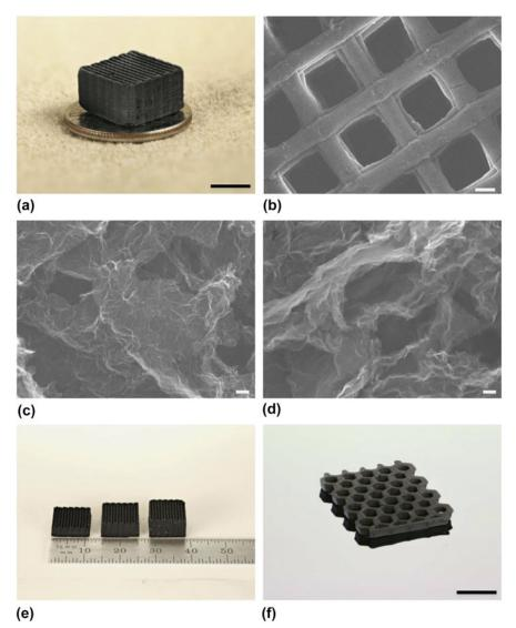
FIG. 10. Morphology and structure of GAs. (a) Optical image of a 3D printed GA microlattice. SEM images of (b) a 3D printed GA microlattice, (c) GA without RF after etching and (d) GA with 4 wt% RF after etching. Optical image of (e) 3D printed GA microlattices with varying thickness and (f) a 3D printed GA honeycomb. Scale bars, 5 mm (a), 200 mm (b), 100 nm (c, d), and 1 cm (f). Reproduced by permission from Ref. 145 (Nature Publishing Group).
