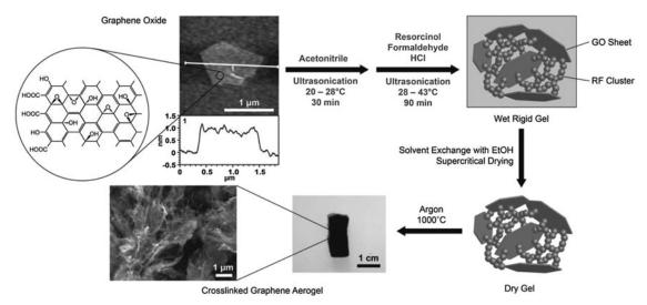
FIG. 5. Diagram of the fast GA preparation process. Reproduced by permission from Ref. 75 (Elsevier).
