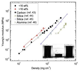
FIG. 3. Dependence of Young's modulus on density for monolithic CNT foams compared to carbon, silica, and alumina aerogels. The inset shows the sequence of uniaxial compression of a monolith  $30 \text{ mg/cm}^3$  and 55 wt% CNT content, illustrating the superelastic behavior with complete strain recovery after compression to strains as large as 76%. Reproduced by permission from Ref. 42 (American Institute of Physics).
