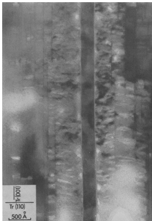
Figure 15. Transmission electron micrograph of Baynton olivine alteration associated with oriented inclusions of late magmatic oxides.
