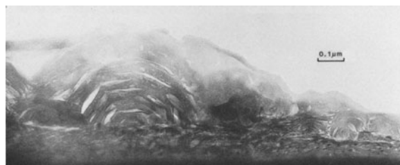
Figure 17. Transmission electron micrograph of halloysite in channel in Townsville olivine; smectite at channel wall.
