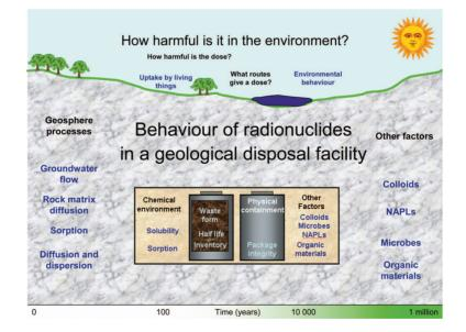
FIG. 1. Behaviour of radionuclides in a geological disposal facility; key features, events and processes. Figure published with the permission of the NDA.
