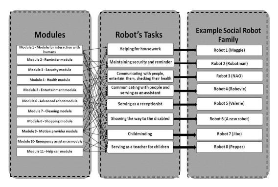
Figure 4. Conceptual structure for a social robot family with behavioural modules
