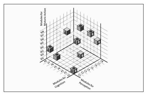
Figure 1. Representation of mechatronic behaviour modules using 3D DSM (Erden, 2018)
