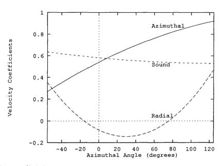
Figure 1. Variations of the velocity coefficients  $q_i$  as functions of the spiral coordinate  $\Psi$  from the post-shock region (left end) to the pre-shock region (right end).  $\Psi = 0$  represents the sonic surface.
