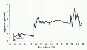
Fig. 5. Dragometer signal. Rapid increase on 15 July 1992 is inferred to be when cable became taut and fish began ploughing through till.
