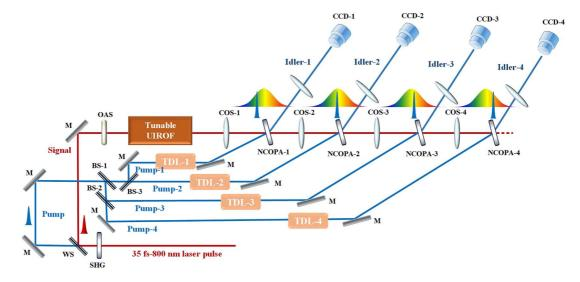
Figure 5. Setup of single-shot ultrafast imaging for the tunable UIROF by NCOPAs. BS-1–BS-3, beam splitters; CCD-1–CCD-4, charge-coupled devices; COS-1–COS-4, confocal optical systems; M, mirror; NCOPA-1–NCOPA-4, noncollinear optical-parametric amplifiers; OAS, optical attenuation slice; SHG, second-harmonic generator; TDL-1–TDL-4, time delay lines; WS, wavelength separator.
