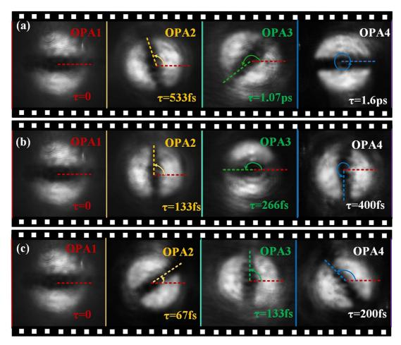
Figure 6. The instantaneous idler images of the rotating ring lattice by the ultrafast real-time frame NCOPA imaging. (a)  $\Omega = 3.95$  Trad/s with the imaging rate of 1.9 Tfps; (b)  $\Omega = 11.9$  Trad/s with the imaging rate of 7.5 Tfps; (c)  $\Omega = 11.9$  Trad/s with the imaging rate of 15 Tfps.
