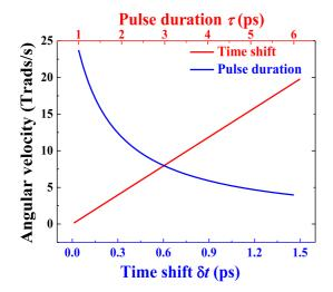
Figure 4. The rotating angular velocity versus time shift and pulse width when  $l = \pm 1$ .
