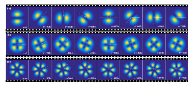
Figure 1. The simulation for the evolution of the interference intensity distribution of a tunable UIROF with (a)  $l = \pm 1$  and  $\Omega = 7.5$  Trad/s; (b)  $l_1 = 1$ ,  $l_2 = -3$  and  $\Omega = 3.75$  Trad/s; (c)  $l = \pm 3$  and  $\Omega = 7.5$  Trad/s.
