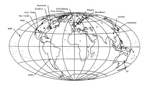
FIGURE I Telescopes available at  $\lambda$ 3mm. Dots without label refer to VLBA antennaes.
