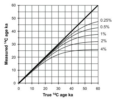
Figure 1 Effect of various levels of open-system behavior with modern carbon on measured  $^{14}\mathrm{C}$  ages.
