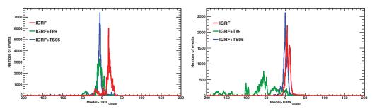
Figure 1. Amount of data as a function of the difference, regarding the component  $B_x$  of the magnetic field, between the model predictions (IGRF alone in red, IGRF+T89 in green and IGRF+TS05 in blue) and the Cluster satellite measurements during 2 - 7 November 2011 (left) and 5 - 9 March 2012 (right).
