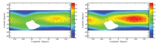
Figure 2. Average upper cutoff computed for the first six months of 2012 selecting particles arriving within  $5^{\circ}$  (left) and  $20^{\circ}$  (right) from the local zenith. The color scale represents the cutoff rigidity in GV. The white region in both maps is the South Atlantic Anomaly region excluded in this analysis.
