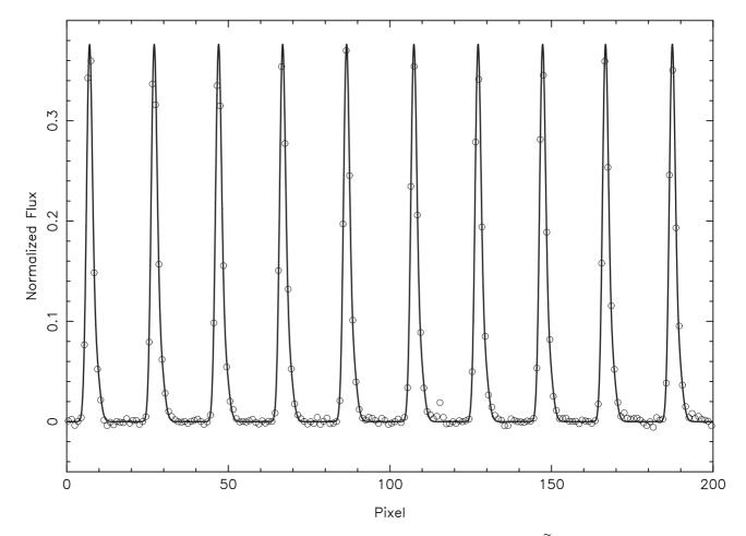
Figure 2 Concatenation of emission lines from a group of fibres (hollow circles, corresponding to the  $\widetilde{F}'$  function). Since there are no dead fibres in this group, ten emission lines were extracted and were used for the fit following the procedure described in the text. The best fit (the F' function) is shown as a thick line and faithfully represents the data. In particular, it reproduces the asymmetric, high-wavelength wing of each emission line.
