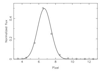
**Figure 7** 8408.2096 Å CuAr emission line extracted from fibre 1 of a CCD2 calibration lamp observation (circles). The emission line is symmetric and can be fitted by a single Gaussian function of internal dispersion  $\sigma = 0.74$  (line).
