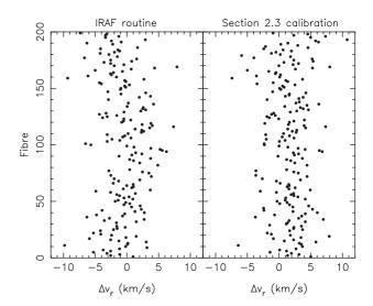
**Figure 6** Difference in radial velocity between the different fibres and fibre 100 for a twilight observation. In the left panel, the spectra were calibrated using the IRAF routine IDENTIFY; in the right panel the calibration was performed using the shape of the LSF, as explained in Section 2.3. The IRAF calibration generates an arc-shaped systematic error that depends on the fibre number while our procedure does not introduce such errors.
