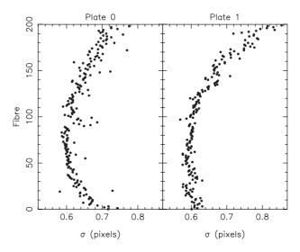
**Figure 8** Evolution of the internal dispersion,  $\sigma$ , of the LSF across CCD2 when fitted by a single Gaussian function as in Figure 7. Although the LSF remains symmetric across CCD2 (contrary to CCD1), its width varies substantially.
