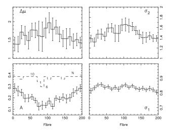
**Figure 3** Evolution of the four LSF-related parameters A (bottom-left panel),  $\sigma_1$  (bottom right),  $\sigma_2$  (top right), and  $\Delta\mu$  (top left) across CCD1. The three parameters representing the perturbation of the LSF  $(A, \sigma_2, \text{ and } \Delta\mu)$  show substantial variations across the CCD. The number of fibres, N, used for the fit is plotted as a thin dashed histogram in the bottom-left panel.
