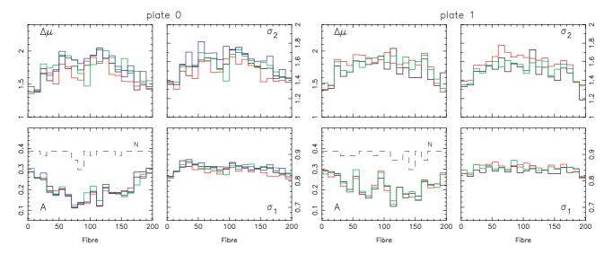
**Figure 4** Same as Figure 3 but with the evolution of the LSF parameters for all the observations that were made during a single night. The parameters for observations on plate 0 are shown in the left panels and those performed on plate 1 are shown in the right panels. Although the parameters evolve in a similar way for all the fits, there are variations with plate and/or observation that prevent us from using a generic set of parameters for the whole night.
