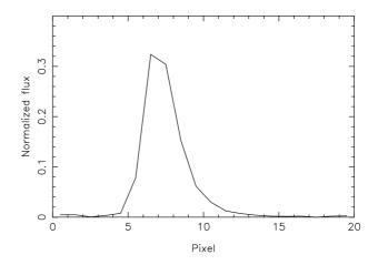
**Figure 1** 5105.541 Å Cu emission line extracted from fibre 1 of a CCD1 calibration lamp observation. The emission line shows an asymmetry towards higher wavelengths that accounts for  $\sim$ 30% of the total signal.
