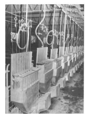
Fig. 2. An automatic frequent feeder for delivering feed at three-hourly intervals.
