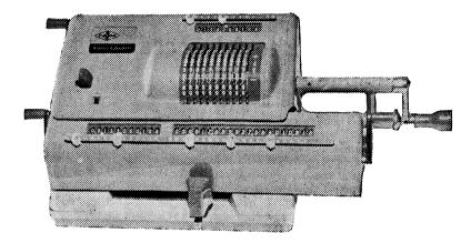
The Nippon Master is a compact, extremely robust hand calculator, encased in high impact resin, which increases protection against damage, and the numeral registers are protected by clear perspex shields.
