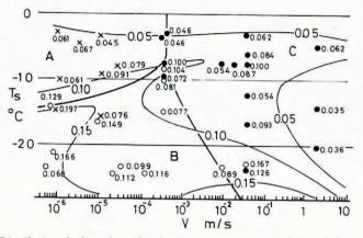
Fig. 4. Distribution of values of  $\mu_k$  plotted against temperatures and velocities (after Huzioka):  $\times$  A-type,  $\bigcirc$  B-type,  $\bigcirc$  C-type.
