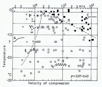
Fig. 5. Modes of fracture of snow columns subjected to uniaxial compression under various temperatures and velocities (after Kinosita): × region A, plastically deformed, ○ region B, interruptedly fractured, ● region C, continuously fractured.
