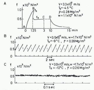
Fig. 3. Three types of oscillograms obtained at different sliding velocities.
