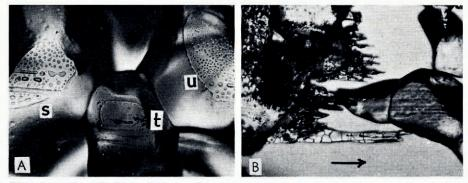
Fig. 6. Photomicrographs of the frictional interfaces between snow and glass and methacrylic resin surfaces (after Huzioka).
