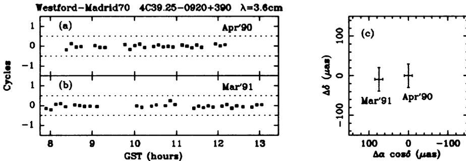
Figure 2. Postfit residuals for the differenced phase delays of the pair 4C39.25/0920+390 at epochs 1990.32 (a) and 1991.22 (b). The position of 4C39.25 relative to 0920+390 at both epochs is shown in (c). The origin corresponds to the position at epoch 1990.32.
