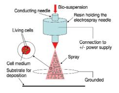
Figure 1. Schematic of the electrohydrodynamic jetting equipment.
