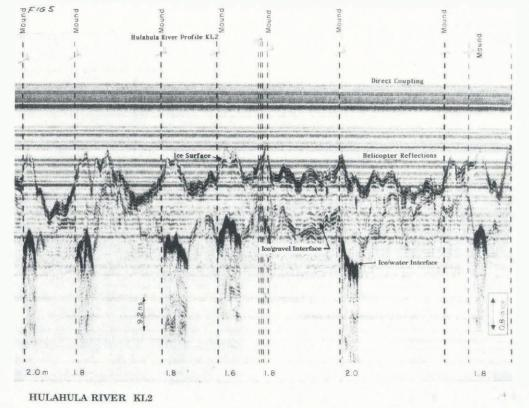
Fig. 3. Short-pulse radar profile taken along the ridges of eight consecutive mounds in Hulahula River. Numbers at the bottom are approximate depths in meters of water under the ridges as interpreted using the ice-depth scale on the graph. "KL2" is one of about 100 such profiles compiled in a CRREL report.
